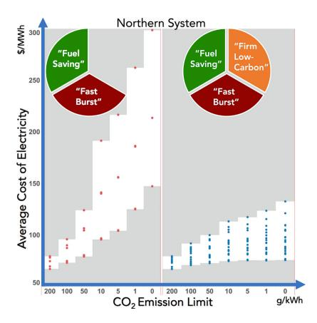
Figure 1: Average Cost of Electricity under Various Technology Assumptions and CO<sub>2</sub> Emission Limits for the Northern System (a) with a decarbonization policy that ex-ante excludes firm lowcarbon resources on the left and (b) with a decarbonization policy that includes firm low-carbon resources on the right.
